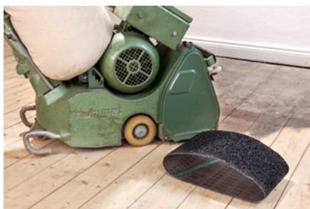
Refurnishment of wooden floors | Belt sander
