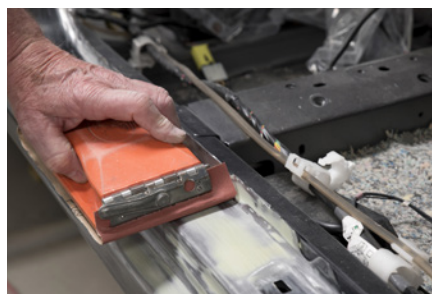
Off-hand grinding - Bodywork
