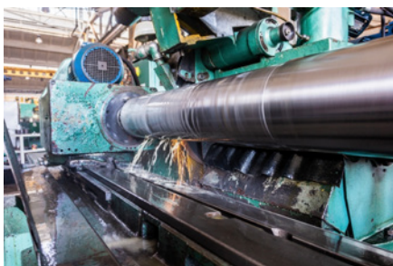
Wet grinding of steel rolls and cylinders
